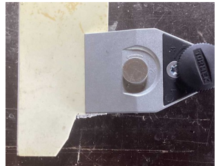
Fig. 2.4: Shaped sheet in jig
